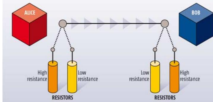
2000 kilometres long, much further than the best quantum key distribution (QKD) devices tried so far. Tests show a signal sent via Kish's device is received with 99.98 per cent accuracy, and that a maximum of just 0.19 per cent of the bits sent are vulnerable to eavesdropping. The error rate is down to the inherent resistance of the wire, and choosing a larger wire in future models should help reduce it further.
