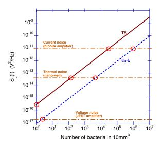
Fig. 2. Estimation of the ultimate limits of detectability of *E. coli* with the tested phages and various measurement arrangements. A linear response is assumed. The various detection limits are indicated by circles where the X coordinate of the center of the circle is the limit.
