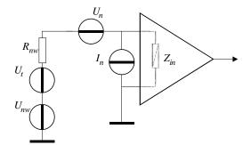
Fig. 1. Simplified noise circuitry of the nano-well arrangement.  $U_{nw}$ ,  $U_t$  and  $R_{nw}$  are the signal voltage generator, the thermal noise voltage generator and the internal resistance (1 MOhm in the experiments) of the nano-well, respectively.  $U_n$  and  $I_n$  are the input noise voltage and input noise current generators of the preamplifier, respectively.  $Z_{in}$  is the input impedance of the preamplifier (100 MOhm in the experiments, thus it can be disregarded).
