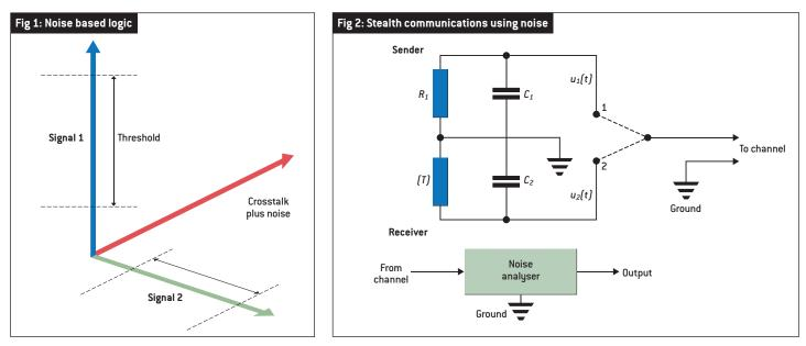
Fig 1: In this scheme, electronic noise is used as the carrier of a logic value. The figure shows noise based logic base vectors, which are orthogonal to each other and to the background noise. Fig 2: This zero signal power communication scheme uses the thermal noise (or Johnson noise) of resistors to data exchange in stealth mode. Information is transmitted using the statistical properties of the modulated noise.
