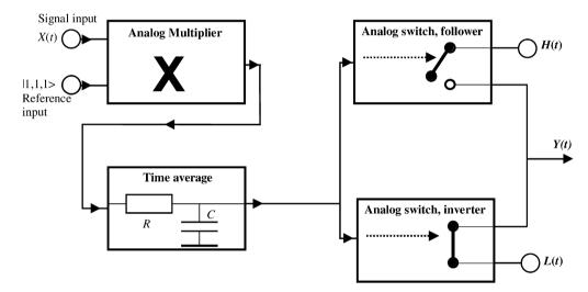
**Fig. 3.** Detecting the component  $|1, 1, 1\rangle$  in the superposition X(t). All the other orthogonal elements need a similar circuitry for detection. L(t) represents the logic value (noise) for "False" and H(t) the logic value for "True".
