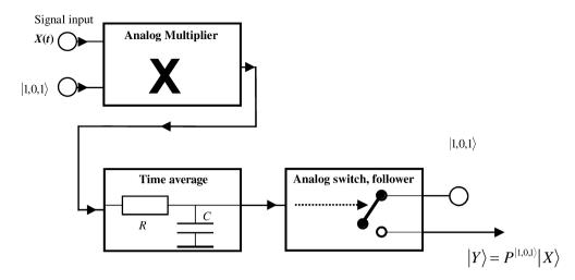
**Fig. 4.** Noise-based logic projection operator  $P^{|1,0,1\rangle}$  for the component  $|1,0,1\rangle$  in the input superposition X(t).
