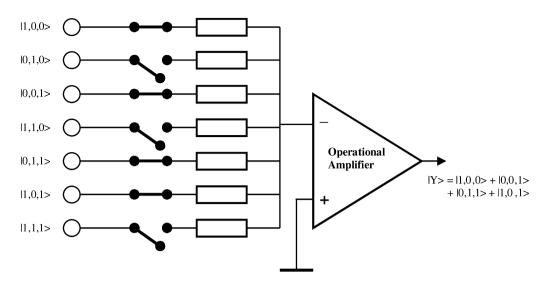
Fig. 2. Example of controlled adder for discrete superpositions made by an operational amplifier. All resistors have the same value.
