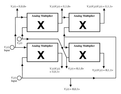
Fig. 1. Making the system of  $2^N - 1$  orthogonal noise-based binary vector states comprising the hyperspace vectors with N = 3.
