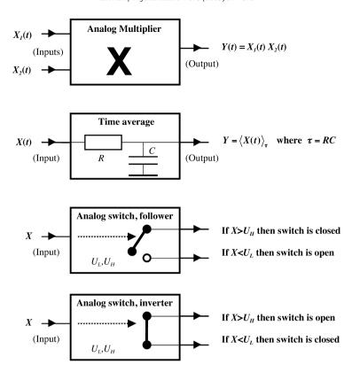
Fig. 2. The analog circuit elements that can be used to realize the gates below. There are some other trivial building elements, such as linear adders and amplifiers, not shown here.
