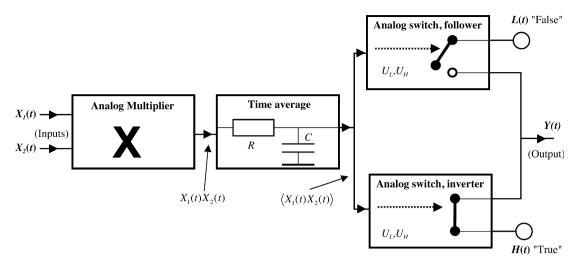
**Fig. 4.** Simple, noise based XOR circuit (binary or multi-value-input). If the two inputs (or arbitrary number of logic values) are equal, the output is *False*, otherwise it is *True*. If the second input is connected to reference H(t), we get an INVERTER gate.
