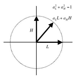
Fig. 1. Vector representation of noise-based logic with two base values. When only single base vectors are used, the logic is binary. If a superposition is used, the logic is fuzzy with continuum values along the unit circle.
