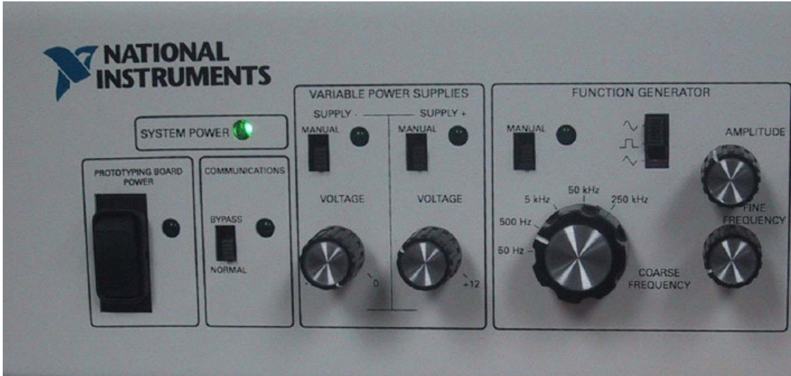
Fig. 2. Front panel of the Elvis bench top.
